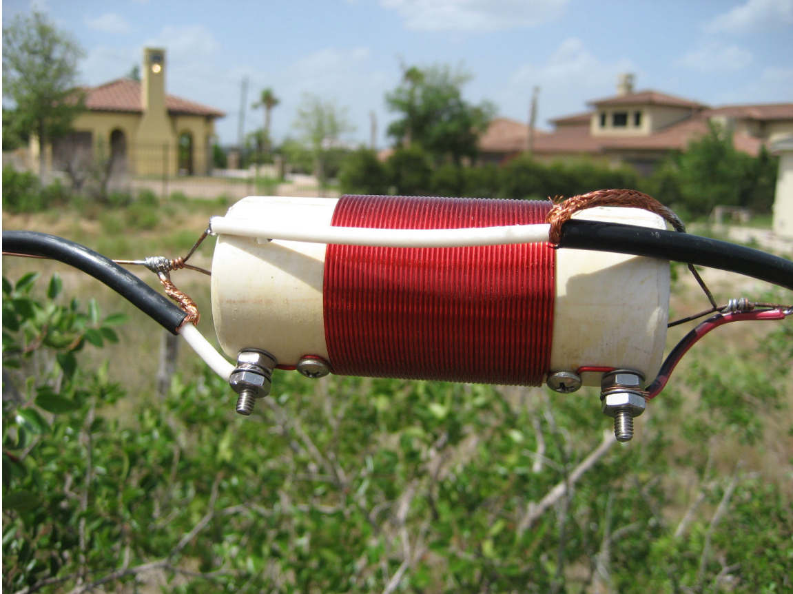
Figure 4. Center of antenna coil and capacitors (RG8x coax).
