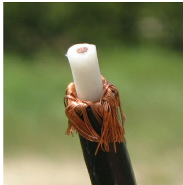
Figure 5. Preparation of the open ends of the capacitors to prevent arcing.
